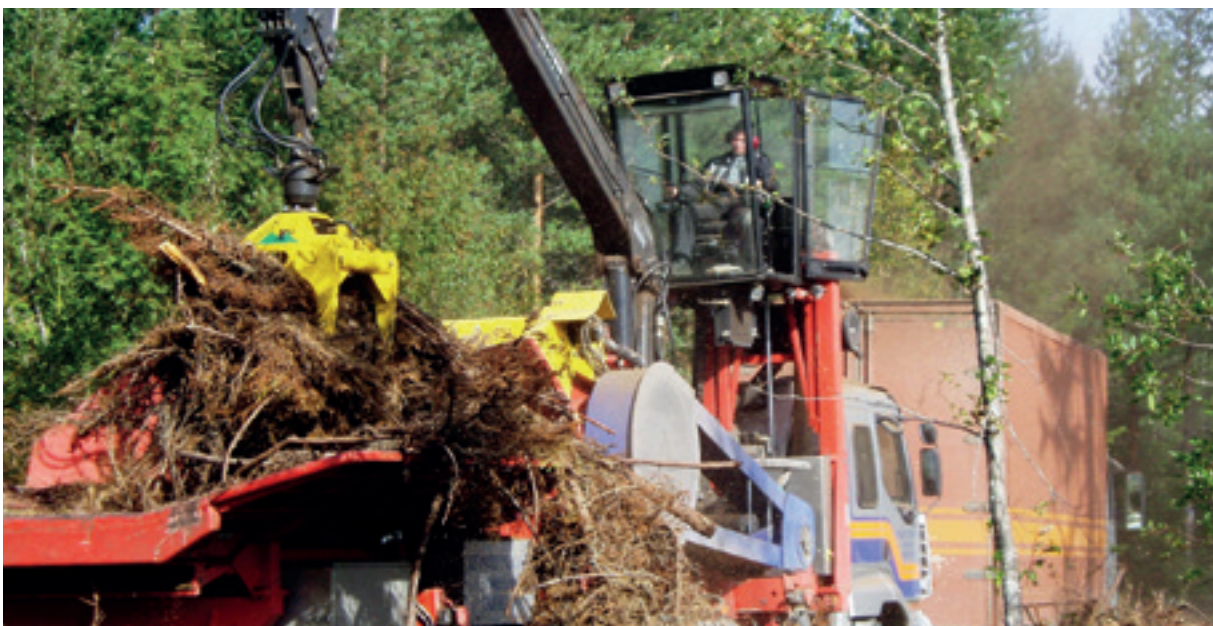
Chipping of logging residues (LHM Hakkurit Oy)
