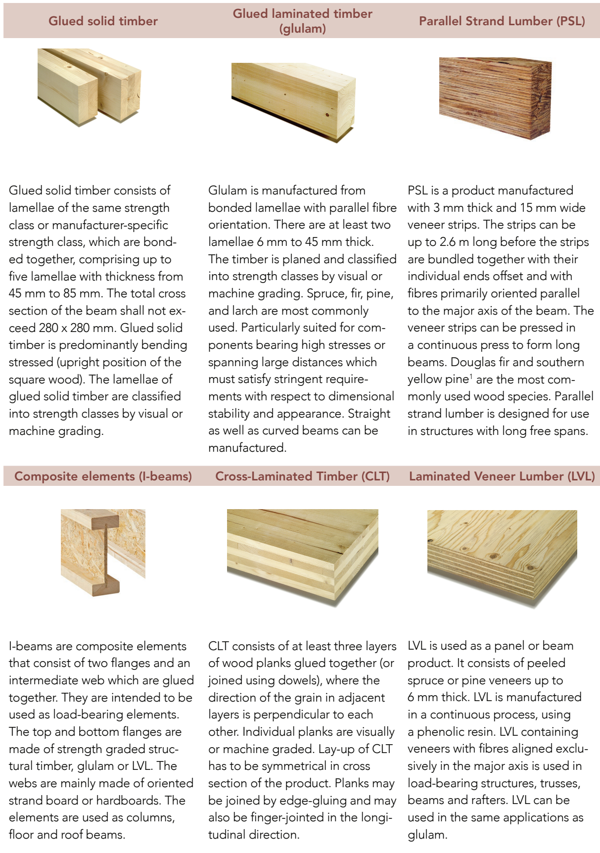
Figure 3.7. Examples of engineered construction materials
