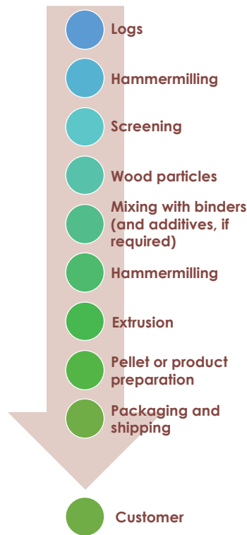
Figure 4.10. Simplified production process of a wood-based composite product
